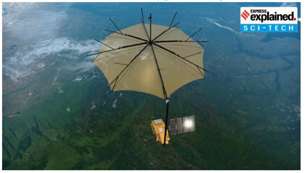
Biomass is the first satellite in the world to host a P-band SAR. The satellite is fitted with a huge 12 m antenna which will be deployed as it begins its sweep over the Earth. (Illustration/ESA)
