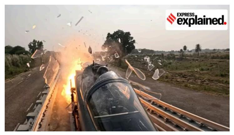
The rocket sled is a ground-based testing system, which is propelled by rockets to climb to high speeds while moving on rail tracks, simulating the aerodynamic conditions of an aircraft in flight. (Ministry of Defence)
