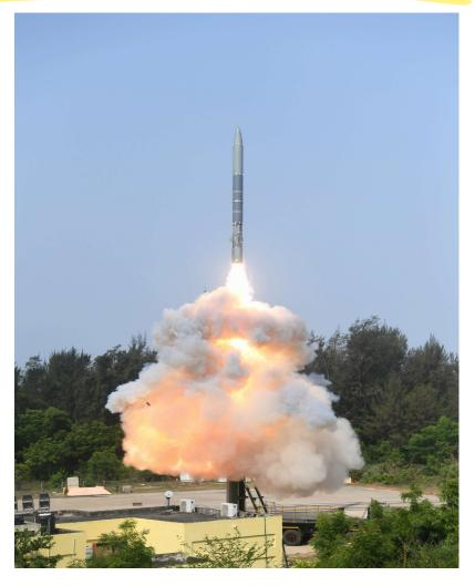
This canister-based missile system consists of several advanced sub-systems, namely two-stage solid opulsion system, electromechanical actuator system, precision inertial navigation system etc. The stem carries advanced light-weight torpedo as payload along with parachute-based release system.
