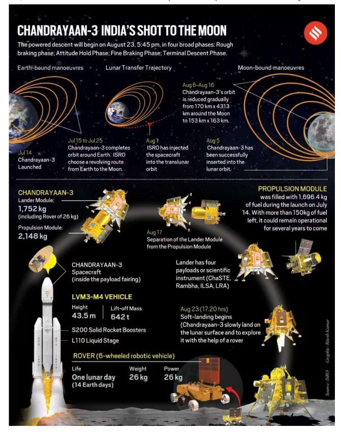
Here's how the Chandrayaan-3 reached the lunar orbit and how it plans to descend to the Moon's surface.
