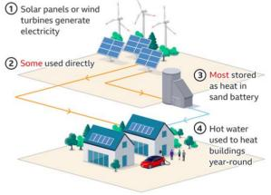
How sand batteries work
