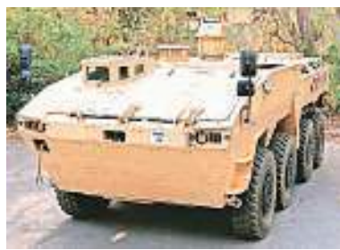
An Infantry Protected Mobility Vehicle jointly developed by TASL and DRDO. Indian Army
